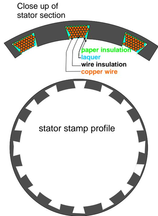
Stator laminate side view with visual example
