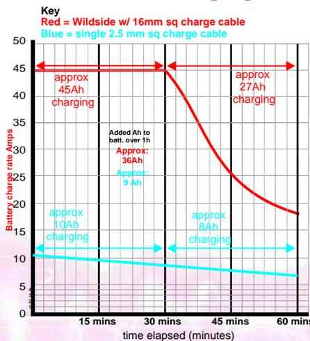
The **Wildside** tow kit has replaced approximately 36Ah of charge into the battery over the 60 minute period which is 4 times more than what was achieved by the 2.5mm sq cable.
